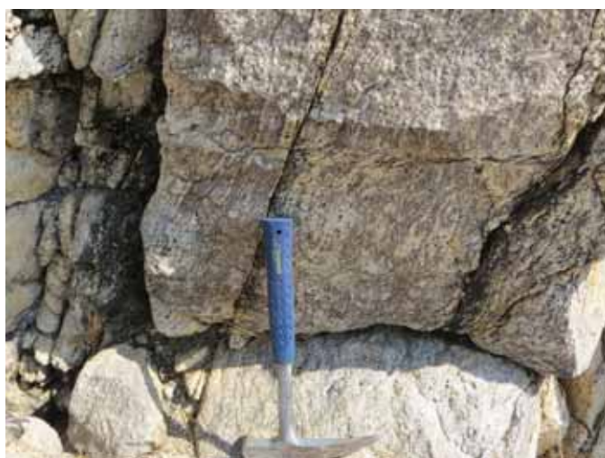
Figure 3: Outcrop of hard, impermeable crystalline rock cut by discrete cracks that will permit water to move through them at depth.
