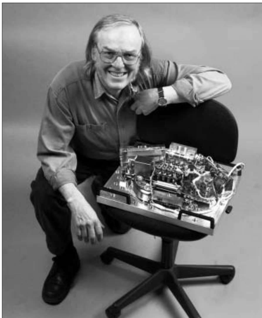
Spin off from the space programme: the miniaturised Beagle 2 mass spectrometer is now being developed for clinical and environmental use.
