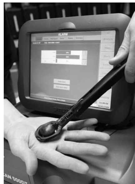
Taking a swab sample to test for possible explosive contamination
