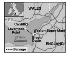
impound the water behind the barrage. As the tide recedes the water would be released through the turbines to generate electricity for a few hours until the tide starts to rise again. The turbines would be generating electricity for about a quarter of the day.
