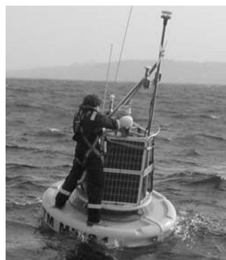
Fig 5: An instrument buoy used to measure salinity at sea.
