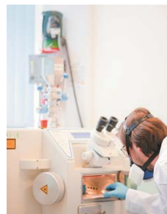
Operating a selective laser melting system
