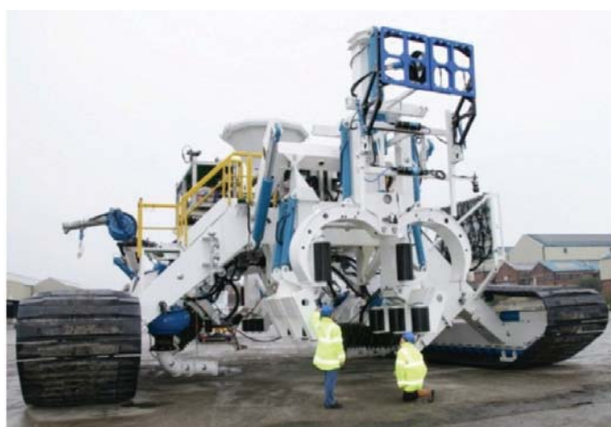
Figure 2: SMD heavy duty remote controlled subsea trenching machine, RT1 – Courtesy of Deepocean Ltd
