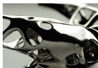
Structurally optimised design, 3D printed in stainless steel
