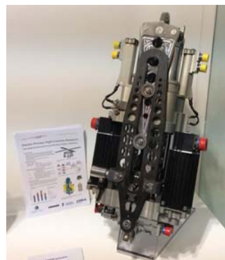
Electromechanical actuator for helicopters developed in partnership with Liebherr Group and Airbus Group Innovations on display on the Clean Sky booth at the Paris Airshow in June 2015
