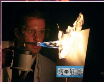
Fig 2 - Silicon carbide electronics under a flame test in the Newcastle Laboratory (the insert at the bottom shows the construction of the sensor and associated electronics).
