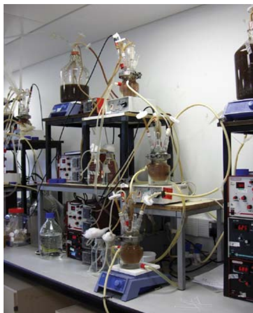
Figure 1. Human colonic model used to simulate the large intestine (and identify mechanisms of prebiotic effects). The model gives a close reflection to in vivo events and is used to plan subsequent human trials. Its use obviates the need for animal experimentation in prebiotic testing.
