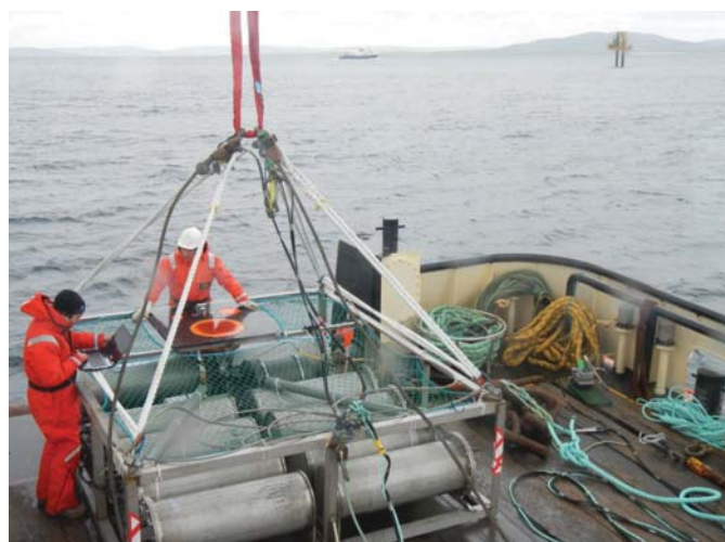
The FLOWBEC sonar frame being prepared for lowering to the sea bed for a 2-week period monitoring marine wildlife at the European Marine Energy Centre tidal test site in 2012. The OpenHydro tide turbine platform can be seen in the top right of the image. Photo by Dr Beth Scott, University of Aberdeen.
