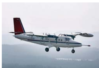
Airborne geophysical surveys require low altitude flying to acquire high resolution data on the subsurface. Image courtesy Tellus Border project, supported by the EU INTERREG IVA Cross-Border programme.
