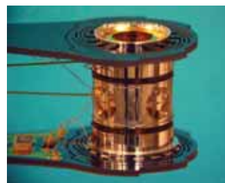
The small gold cylinder, just 8.4mm long, which holds the fuel capsule
