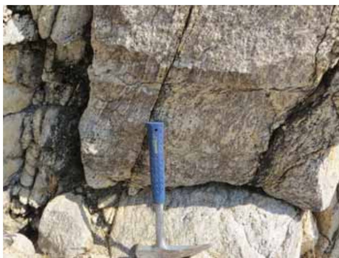
Figure 3: Outcrop of hard, impermeable crystalline rock cut by discrete cracks that will permit water to move through them at depth.
