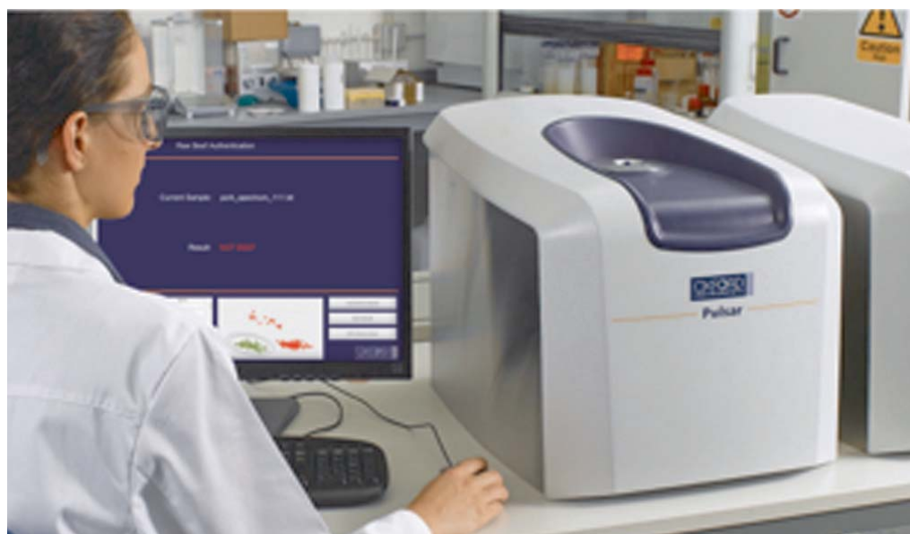
The Pulsar bench-top spectrometer running the IFR-developed beef authentication software
