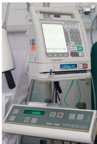
Two different infusion devices delivering medication to one patient in hospital. These devices are programmed by nurses; they should be designed to maximise patient safety (minimising the likelihood of the user programming the wrong rate or volume of medication) – eg, by having consistent interfaces and intuitive user interaction.
