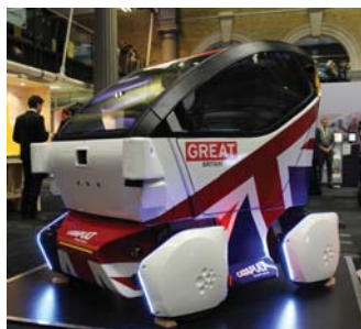
2 seater electric powered automated vehicle pod equipped with sensor and navigation technology from the University of Oxford - part of the LUTZ Pathfinder project from Coventry based company RDM.
