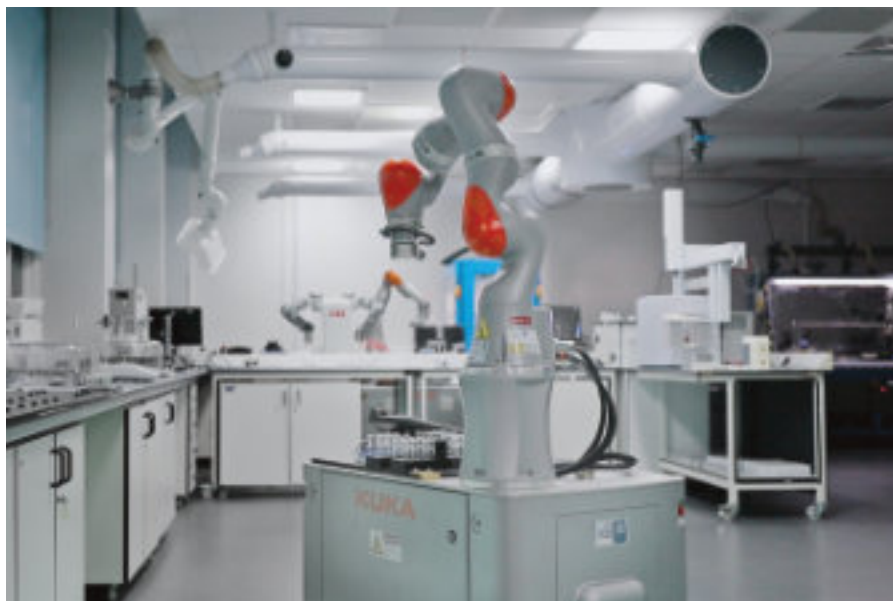
Figure 2: The mobile robotic chemist developed at the University of Liverpool – a physically-embodied AI agent for laboratory R&D problems
