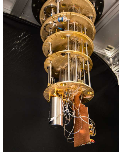
Left to right: Jim Al-Khalili and some young quantum enthusiasts; The IOP's event at the Royal Institution; A multi-stage dilution refrigerator used for cooling superconducting quantum processors to millikelvin temperatures, with layered gold-plated plates and wiring for qubit control and readout (photo by permission of National Quantum Computing Centre)
